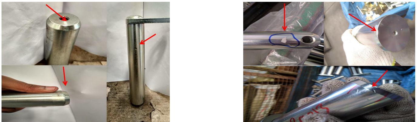
Figure 5: Dents on different components
