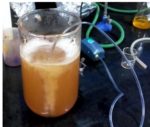
Fig. 1 Glass Reactor with bubbler for Fenton process
