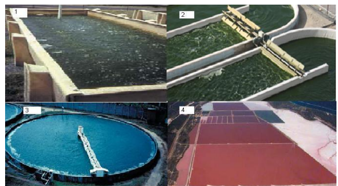
Fig 2. Open System (1) unstirred pond, (2) raceway pond, (3) circular pond
