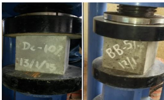
Fig. 3. Shows the of concrete Cubes before Testing
