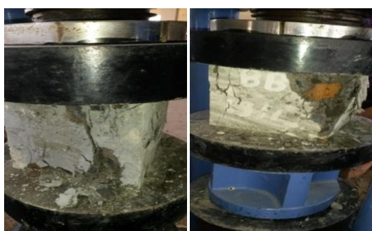
Fig. 4. Shows of concrete Cubes the After Testing
