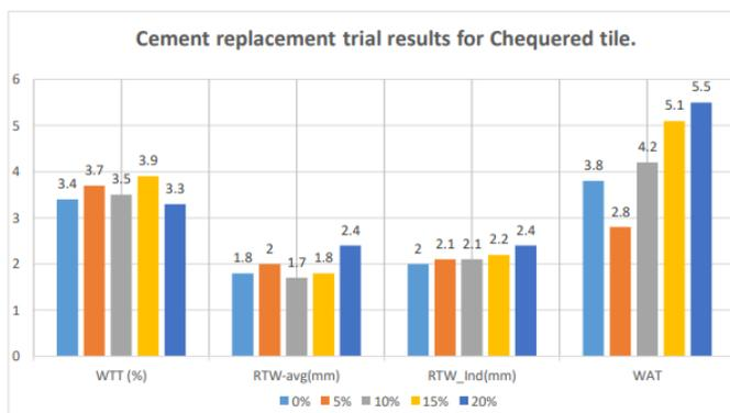
Percentage water absorption and resistance to wear are two of the most prominent characteristics that determines the quality of chequered tile. It is found that even after replacement of cement up to 20% with red mud, all the values obtained for parameters are much within permissible limits as per IS:13801-1993.
