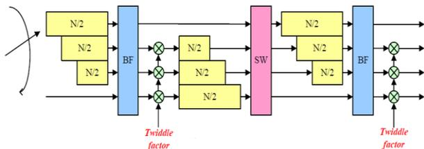
Fig.4. The two stages of N-point R4MDC Architecture
