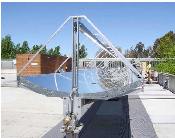
Fig.3. Prototype CHAPS collector at ANU
