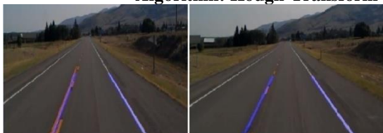
Fig.6: Snapshot of output of lane detection using Hough-transform method
