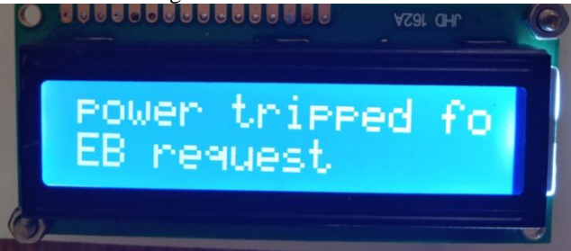
Fig 14 Image of power tripped when electric bill is not paid.
