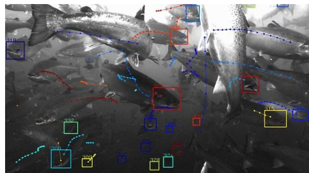
Fig.5Fish density recognizing through AI Waterproof PI Camera
