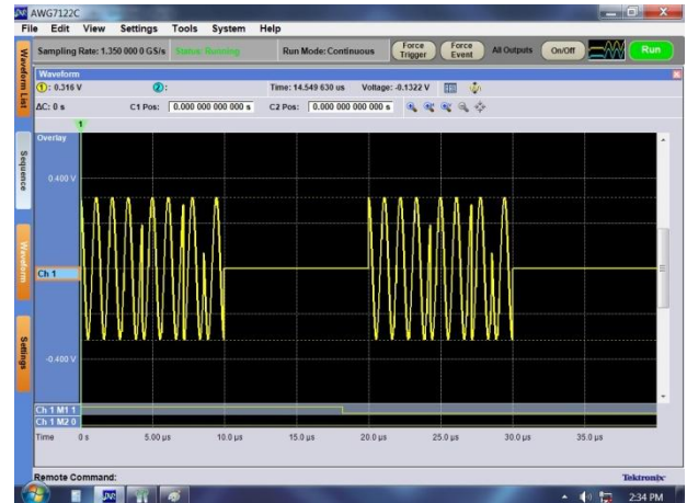
Fig 1: 7 Bit Barker signal generated from the AWG
