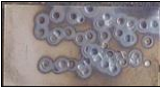
Fig. 4 Spot Weld Quality before Integrating Load Cell
