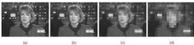
Fig.6. (a) n = 1, original image. (b) n = 4. (c) n = 8. (d) n = 16. Original and corresponding low resolution images. Each square cell consists of n x n pixels in which the intensity of each pixel is replaced by the average intensity of the pixels in that cell.
