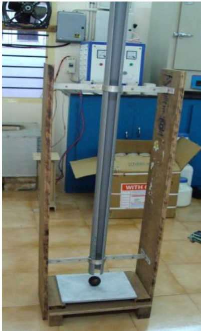
Fig 9: Arrangement for Impact resistance Test
