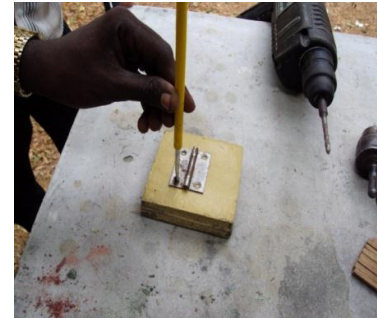
Fig 15: RPC is nailable & Screwable
