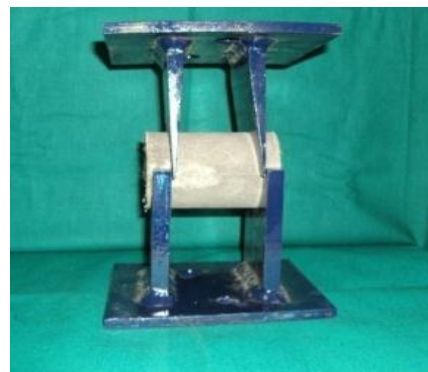
Fig 7: Testing arrangement for Shear strength
