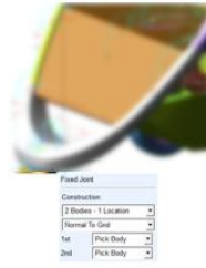
Fig 3: Fixed Joint Connections
