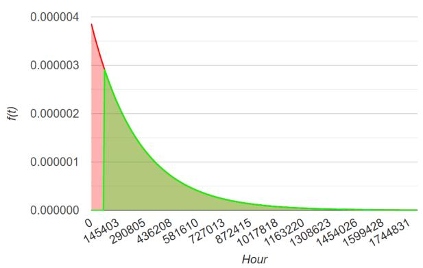
The reliability at 69,000 hours is 0.77, as represented by the green shaded area to the right of the 69,000 hour point in the probability density function (pdf) plot shown above. The unreliability or probability of failure is 0.23, as represented by the pink shaded area to the left of the 69,000 hour point in the pdf plot.
