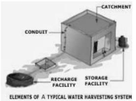
Figure 1: Components of Rainwater Harvesting system
