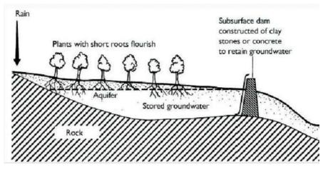
Figure 8: Subsurface Dam
