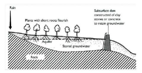
Figure 8: Subsurface Dam
