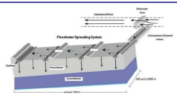
Figure 3: Spreading Basins
