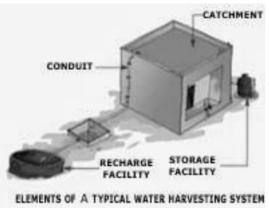
Figure 1: Components of Rainwater Harvesting system
