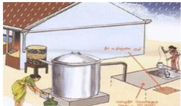
Fig. 7 rain water storage
