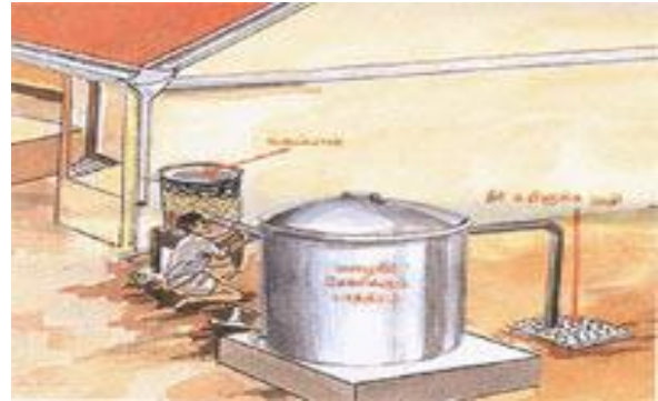
Fig. 5 rain water collected in gutter
