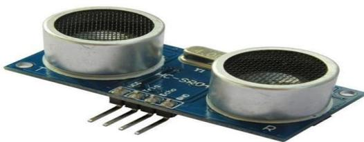
Fig.2. Ultrasonic sensor HC-SR04
