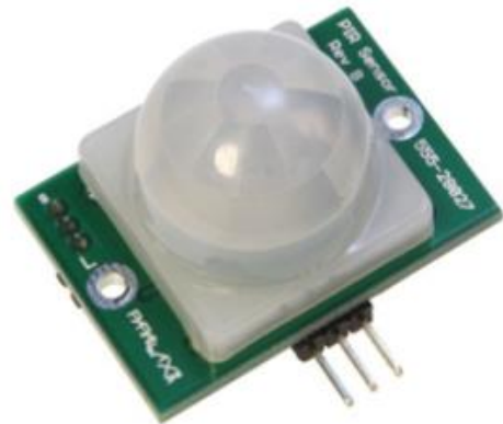
Figure PIR sensor
