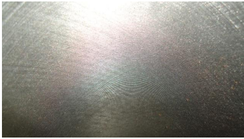
Fig 6.1.2 Defective part with Inner diameter unclear surface
