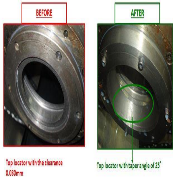
Fig 6.1.5 By providing taper angle 25° top locator at fine boring operation
