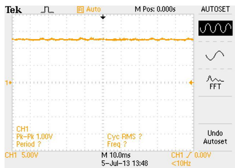
Fig.13. Regulated output voltage of the converter
