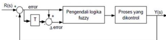
Figure 10. Fuzzy Control Structure.
