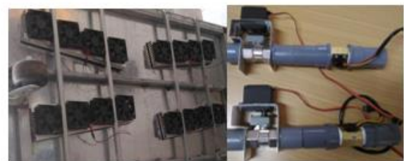
Figure 14. Peltier, flow sensor and DC valve control.
