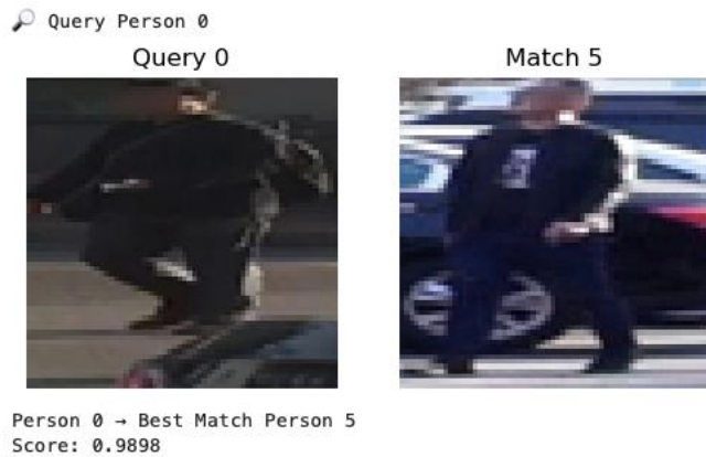
Fig 6. Samples of output results with query images and their best matches with the highest similarity scores.
