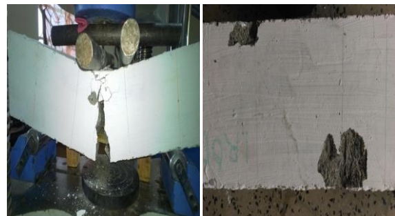
Figure 6: Failure of Concrete Beam
