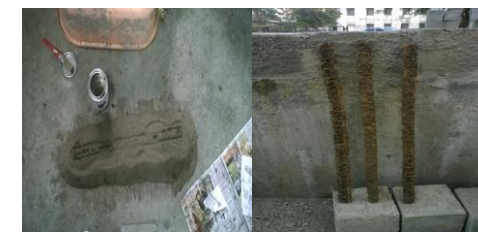
Figure 1: Application of Resin, drying strips, sand application, chicken wounding around strip, and final drying of Bamboo Strip
