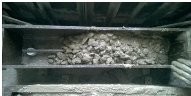
Figure 4: Beam with a Single TMT Steel Rod
