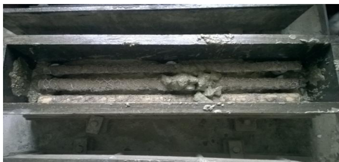
Figure 2: Beam with 6 Bamboo Strips (1/4 th )
