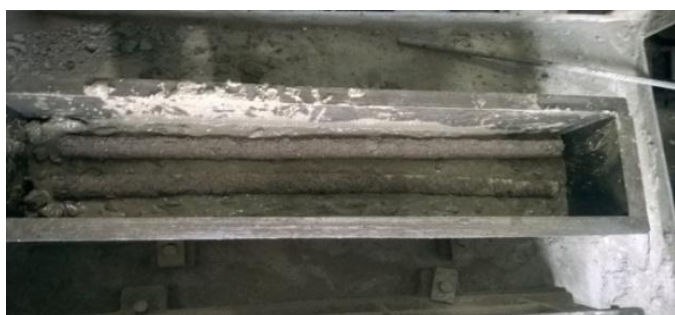
Figure 3: Beam with 4 Bamboo Strips (1/4 th c/s)
