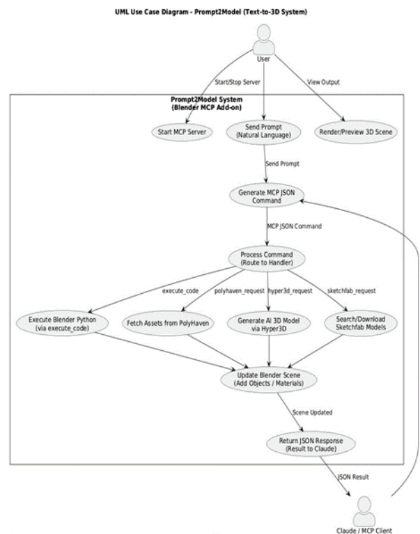
Figure 2: Use Case Diagram representing the various use cases formulated based on UML notation and their interaction between actors and objects. Actors and objects consist of user, Prompt2Model Blender Add-on, and Application client (Claude/MCP).
