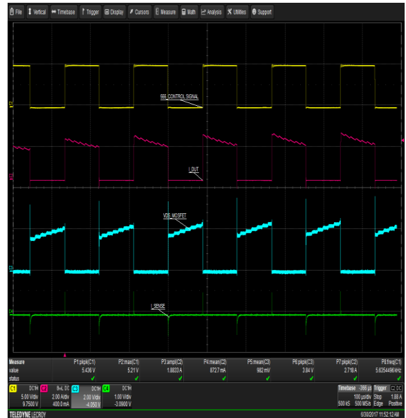
Fig.6 Load transient waveforms of DC Electronic load
