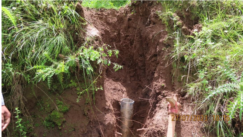
Photo-1: Undisturbed soil sample collection in GI pipe after removal of top organic layer
