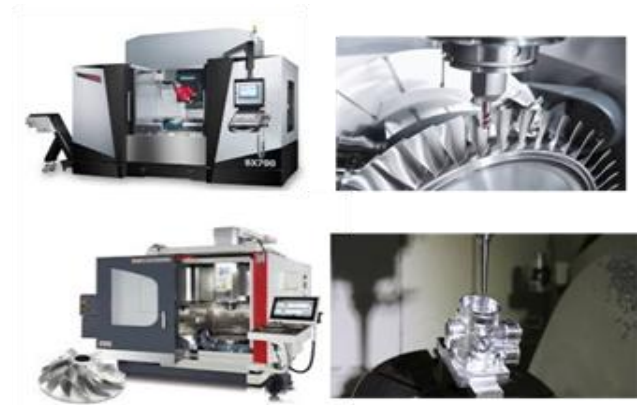
Fig 4:- Multi-axis high-end CNC machine
