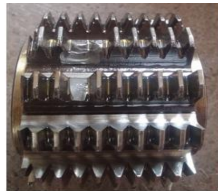
Fig. 7 Failure of Hob Tool
