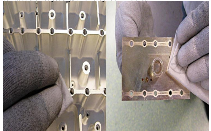
FIG 2. Cleaning the contact surfaces with alcohol. Use clean, lint-free cloth.
