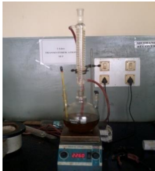
Fig .4 Transesterification set up
