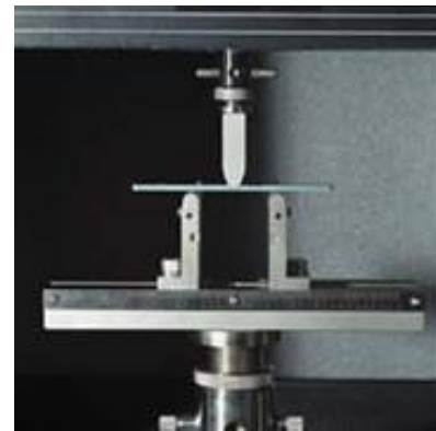
Figure 5: Three point bending specimen
