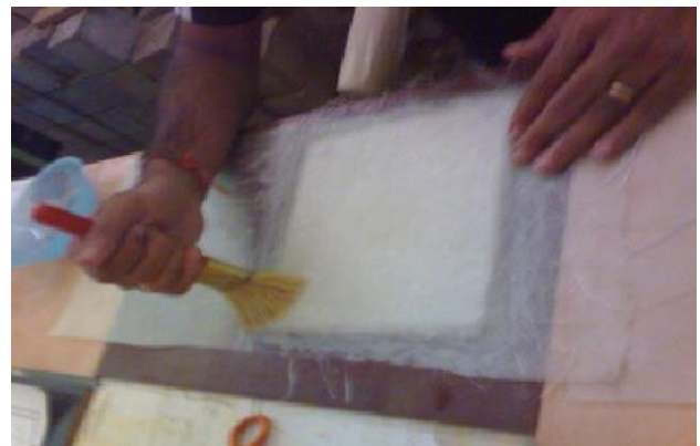
Fabrication of GFRP by hand layup
