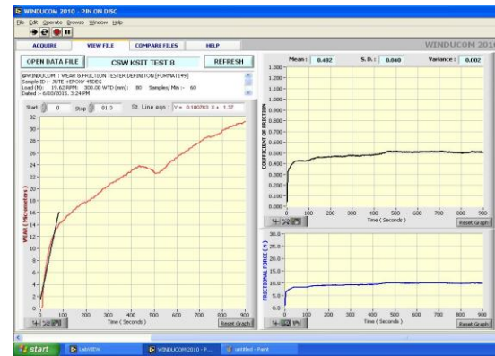
Fig 16 shows the variations in wear, co-efficient of friction, frictional force for 30° orientation for 20N load.
