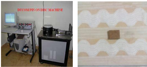
Figure 8 Pin on disc Wear testing machine and specimen
