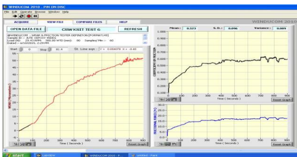
Fig 14 shows the variations in wear, co-efficient of friction, frictional force for 45° orientation for 30N load.
