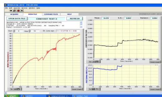
Fig 11 shows the variations in wear, co-efficient of friction, frictional force for 90° orientation for 30N load.
