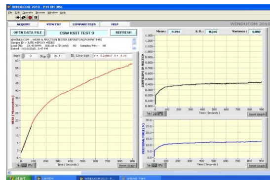
Fig 17 shows the variations in wear, co-efficient of friction, frictional force for 30° orientation for 30N load.
