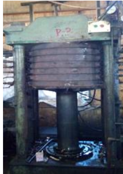
Fig. 8. Tire Curing Machine
