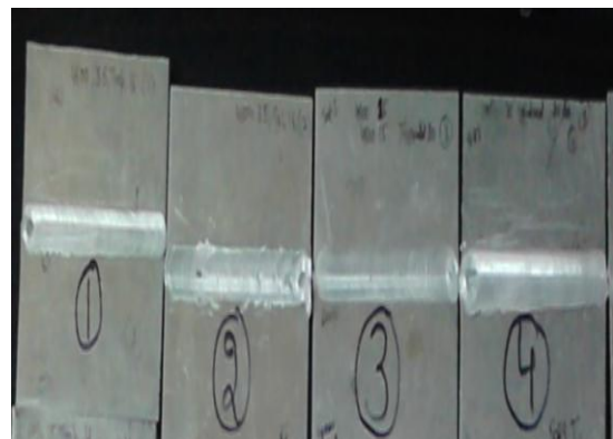
Fig.5 AA Plates after welding
