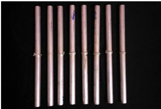
Fig 3. Friction Welded Specimens for Tensile Test
