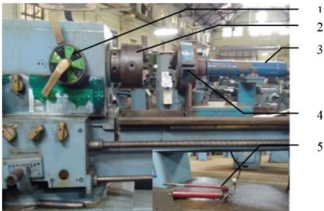
Fig 1. Friction Welding Setup (1.Gear Mechanism 2.Rotating chuck 3.Piston Arrangement 4.Non-rotating Chuck 5.Hydraulic Hand Pump)
