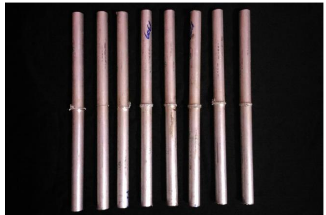
Fig 5. Friction Welded Specimens for Torsion Test
