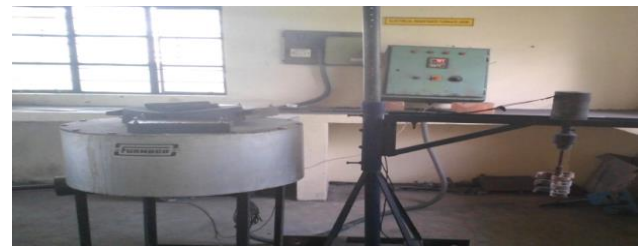
Fig1: Stir casting apparatus
