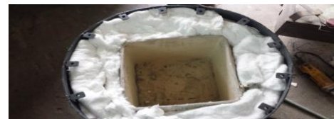
Fig.4.7. Preparation of furnace body diagram
