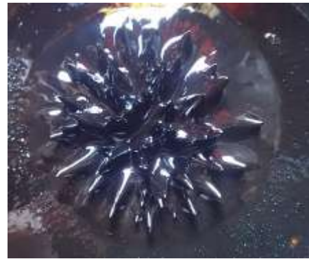
Fig. 7 - Response of the ferrofluid in the presence of the external magnetic field.
