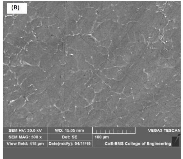
Fig.2.b. Micrograph of Al6061-ZrO<sub>2</sub> particulates with 3wt. % of ZrO<sub>2</sub>
