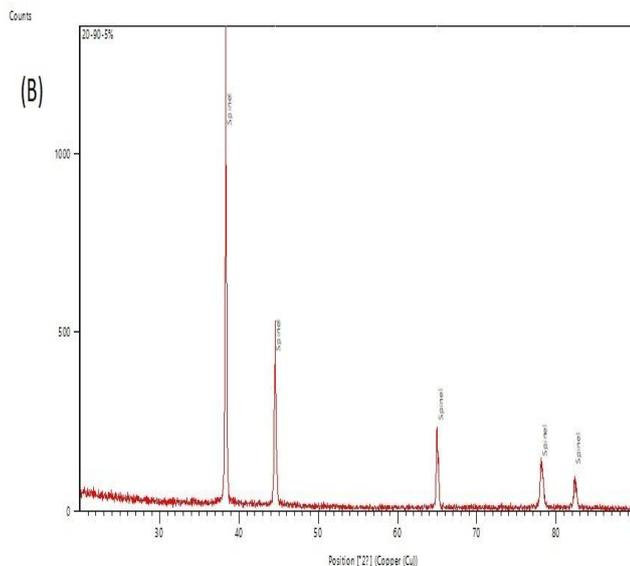
Figure 3.b. XRD pattern for Al6061-ZrO<sub>2</sub> with 5 wt. % ZrO<sub>2</sub>.
