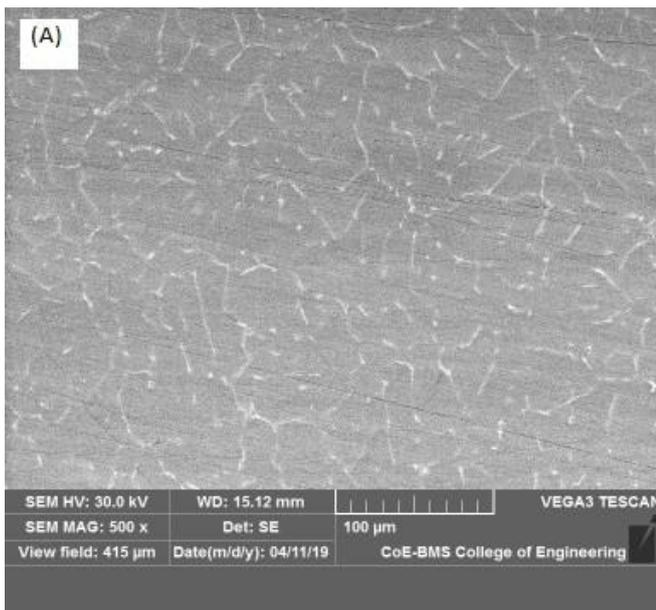
Fig.2.a. Micrograph of Al6061-ZrO<sub>2</sub> particulates with 1wt. % of ZrO<sub>2</sub>
