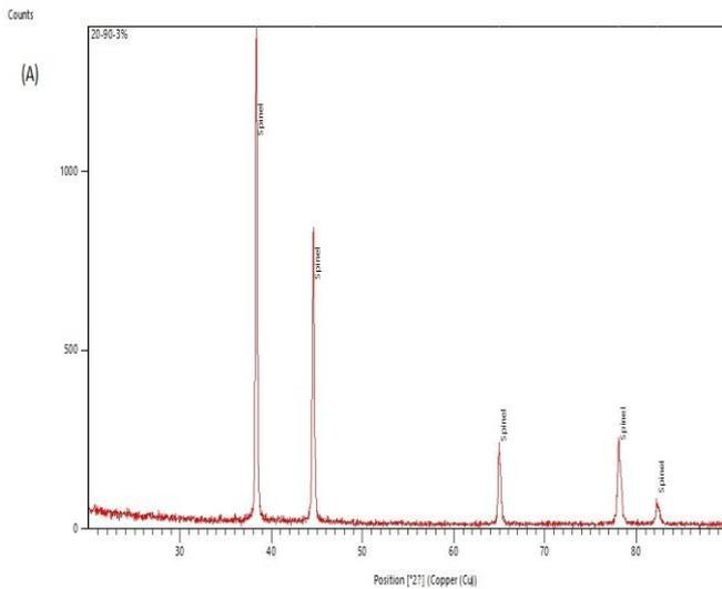
Figure 3.a. XRD pattern for Al6061-ZrO<sub>2</sub> with 3 wt. % ZrO<sub>2</sub>.
