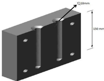
Fig 1. Steel Mould used for casting
