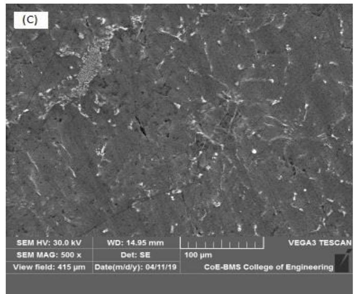
Fig.2.c. Micrograph of Al6061-ZrO<sub>2</sub> particulates with 5wt. % of ZrO<sub>2</sub>
