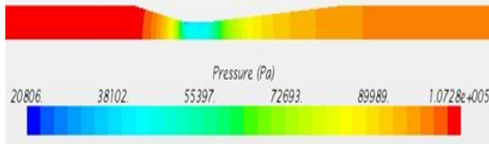
Fig-4.4b. Venturi Pressure Contours.
