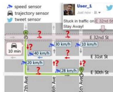
Fig. 1. Problem setting. Our goal is to predict the traffic speed of specific road links, as shown with the red question marks, given: 1) Some speed observations collected by speed sensors, as shown in blue; 2) trajectory and travel time of OD pairs. Note that speeds of passed road links are either observed or to be predicted; 3) tweets describing traffic conditions. Note that the location mentioned by a tweet may be a street covering multiple road links.
