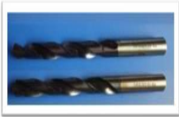
Figure-2: HSS 16mm Drill Bit
