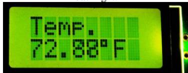
Figure 8: Temperature display. It's an 8x2 character LCD with green backlight.
