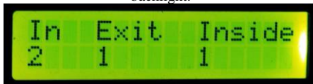
Figure 9: No. of persons count display. It's a 16x2 character LCD with green backlight.
