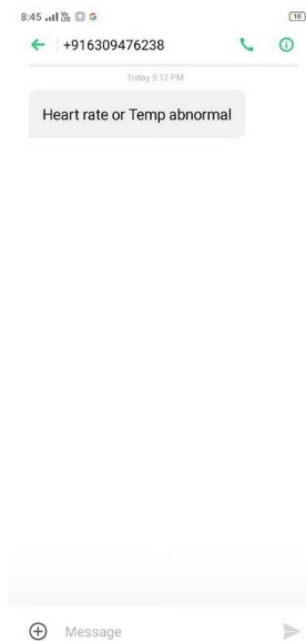
Fig. 7. SMS received on the test handset. Six seconds from threshold crossing to delivery in this instance. Campaign of 23 triggered alerts over 18–25 March 2025: every one delivered, latency range 4.2–11.7 s.
