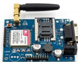
Fig. 5. SIM900A GSM module. All four domestic carrier bands supported. Data attachment disabled at init. Five SMS alerts delivered with zero data balance on 24 March 2025 at 16:20 IST.
