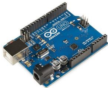
Fig. 1. Arduino UNO R3. Second microcontroller, chosen after the ESP32 heap-crashed at 14:23 IST on 17 February 2025. Runtime memory tracked via freeMemory() every 50 ms throughout development.
