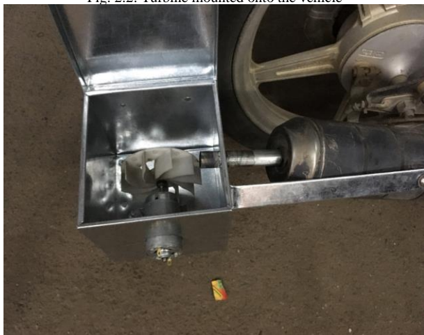
Fig. 2.3: Close up view of Turbine Mounting
