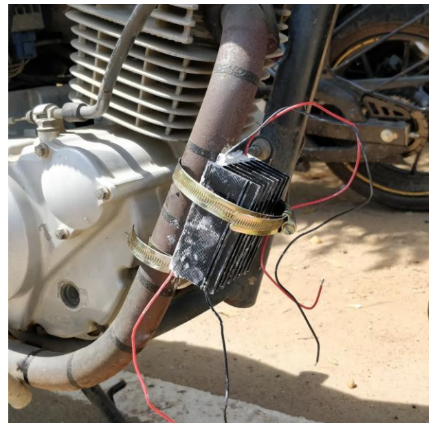
Fig. 2.2. Close up view of Peltier module setup mounted onto the silencer
