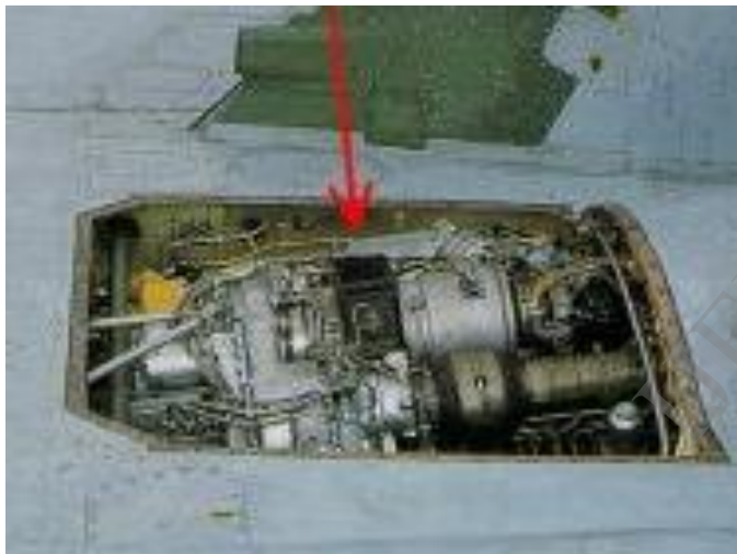
Figure-2 Panel access/position of GTSU (indicated by red arrow) on aircraft.
